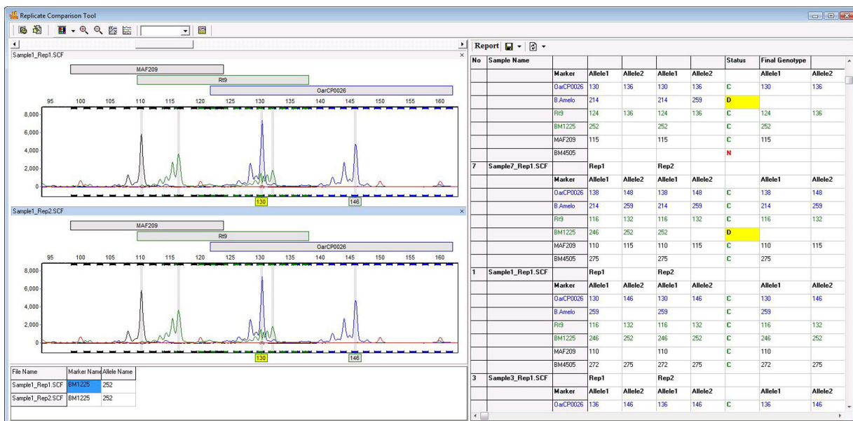
Figure 1: Overview of the Replicate Comparison Tool. Replicates are grouped together and compared in the electropherogram to the left. Allele calls for each replicate are compared to the right; differences are highlighted with yellow flagging.
