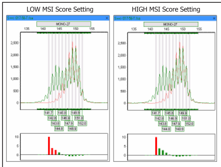
Figure 2. When the MSI Score threshold is lowered, more peaks are identified as instable (red histogram bars). As the MSI Score threshold is increased, only the most relevant peaks are identified as instable.
