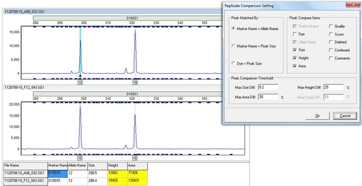
**Figure 2:** Use the Replicate Comparison Settings window to choose which parameters to compare for each replicate. For some parameters (size, area, height, and score) the user may set a range of allowable values.
