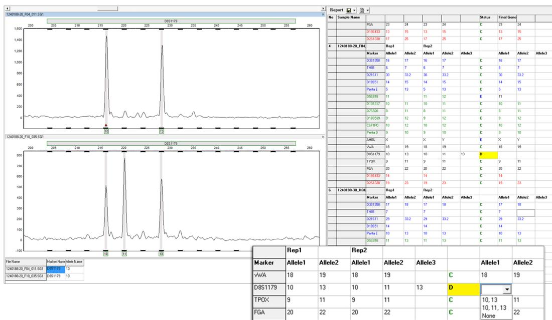
**Figure 4:** The report table. When the program detects a discrepancy between two replicates, the errant marker is flagged and the status column is filled with a D, for discordant. The user may manually choose the call for that locus using a dropdown menu.
